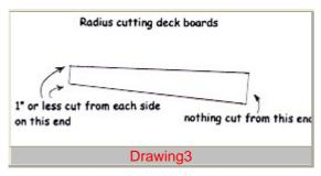
To achieve the desired curve the decking will be trimmed into wedge shaped pieces following the radius of the curves. Cut the 5/4 " decking along it's length tapering from one end to the other. Reference Drawing 3. Trim more from some pieces and less (or none) from others. The sharpness of the radius determines how much to cut.
